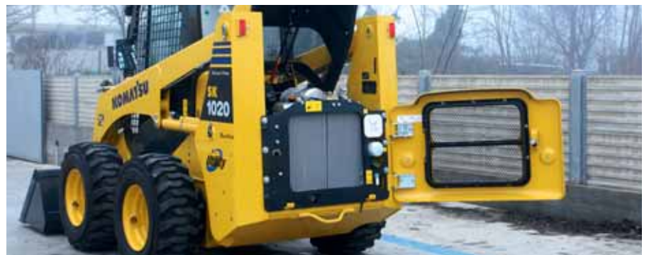
The hatchback: simple inspection and cleaning of the radiators
