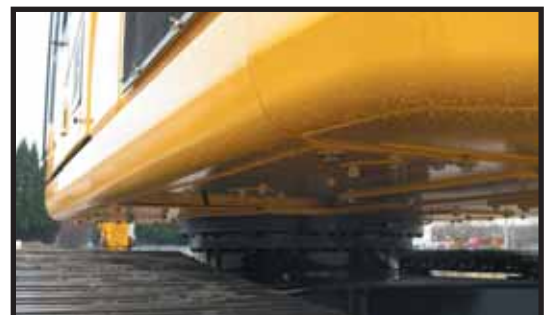
Heavy duty undercovers are fitted to the upper structure offering enhanced resistance to damage from debris on the ground.
