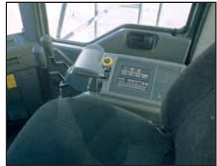
EDIMOS II maintenance monitor panel
