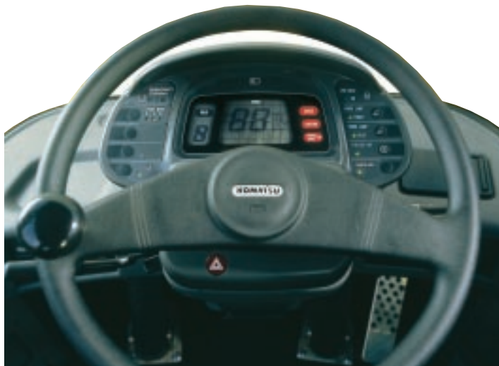
Ergonomically designed main monitor.
