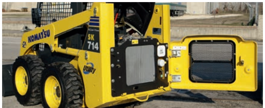
The hatchback: simple inspection and cleaning of the radiators
