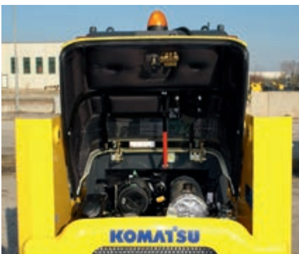
The bonnet: quick engine check
