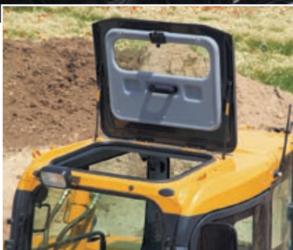
Opening skylight for overhead visibility
