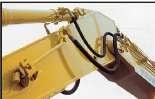
Additional hydraulic circuits
