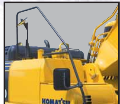
Large handrail for safe access
