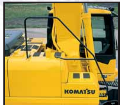
Large handrail for safe access
