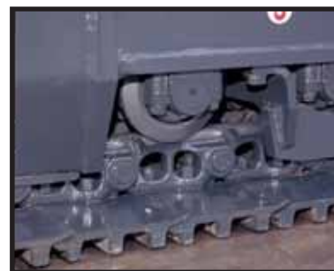
Track link with strut The PC240-7 uses track links with struts, providing superb durability
