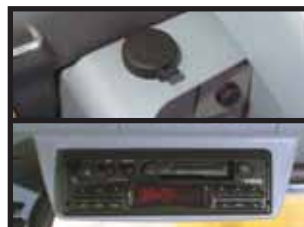
12-Volt power supply and (optional) radio cassette
