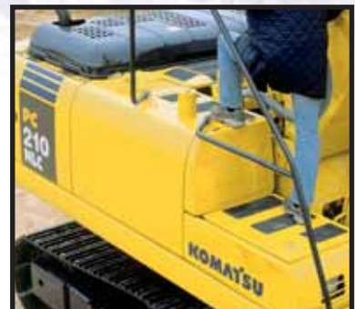
Large handrail for safe access
